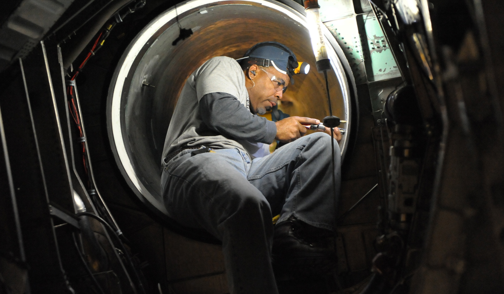
Anthony Farrow, 561st Aircraft Maintenance Squadron Production Support, changes intake fasteners on an F-15 during programmed depot maintenance at Robins Air Force Base, Georgia, in 2016. USAF/Ray Crayton.
